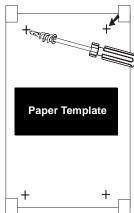
2. Using an electric drill, drill a 3/16inch hole at each of the bottom marks.
